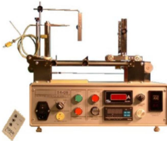
**T4-08M GLOW WIRE TEST APPARATUS WITH MOTOR DRIVE** is intended for testing the flammability and ignitability of components and materials. It is constructed in compliance with IEC (e.g. **60695-2-10, 695-2-1, 335-1, 1058-1, 742, 669-1.**) and also includes electronic feed back heating current stabilizer - regulator, A-meter, thermometer, motor drive and timer.
